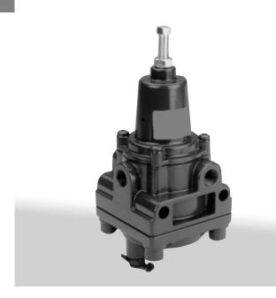
Mechanical Specifications Mounting Pipe or through body Weight 1.6 lb (725 g) Port Size (In, Out, and Gauge) 1/4" NPT Materials of Construction Body: Die-cast aluminum alloy, Irridite and baked Epoxy finish Filter: 3 micron Phenolic impregnated Cellulose Diaphragm: Nitrile Elastomer and Nylon fabric Valve Seat Plug: Nitrile Elastomer Additional Materials: Brass, Zinc plated steel, Acetal
