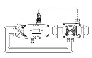
Fig. 4-8: Double acting rotary actuator (YT-2501R)
