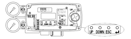
Fig. 9-2: Limit switch type
