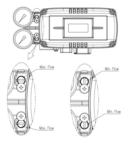
Fig. 6-3: Variable orifice adjustment
