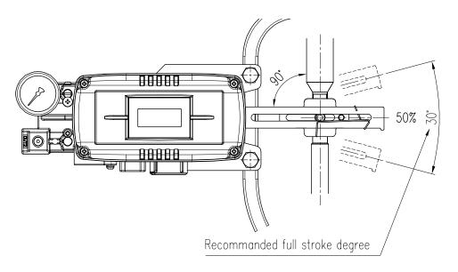
Fig. 3-8: Feedback lever and valve stem
