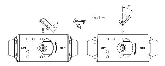
Fig. 3-17: Counter-clockwise and clockwise rotation.
