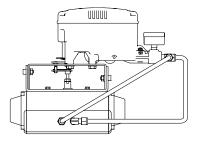
Fig. 4-5: Double acting linear actuator (YT-2500L / 2550L) Fig. 4-6: Double acting rotary actuator (YT-2500R / 2550R)
