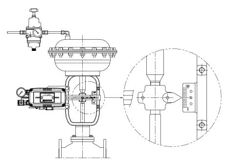
Fig. 3-6: Supplying proper regulated air to the actuator to position the value at 50 %
