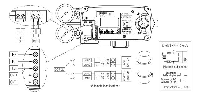
Fig. 5-3: Terminal of two Inductive Proximity Limit Switches (Only YT-2500 / 2550)
