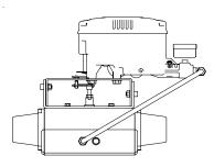
Fig. 4-2: Single acting rotary actuator (YT-2500R / 2550R)
