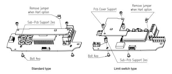
Fig. 7-2: Installation of Optional sub-PCB on Main PCBs
