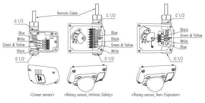
Fig. 5-4: Remote sensor and cables (Only YT-2501)
