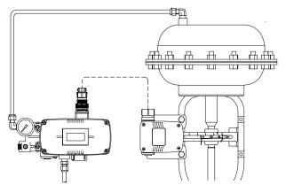
Fig. 4-3: Single acting linear actuator (YT-2501L)
