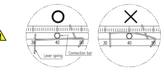
Fig. 3-7: Proper way to insert connection bar between feedback lever and lever spring
