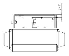
Fig. 3-18: Height to the bracket (fork lever type)
