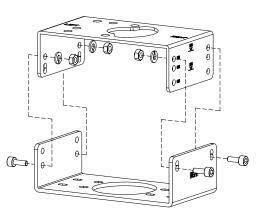
Fig. 3-16: Exploded Brackets
