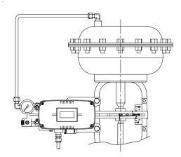
Fig. 4-1: Single acting linear actuator (YT-2500L / 2550L)
