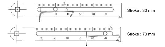
Fig. 3-9: Feedback lever and location of the connection bar
