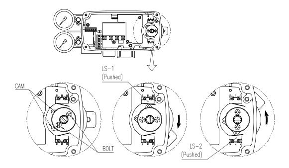
Fig. 6-1: Mechanical Type
