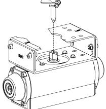
Fig. 3-19: Main shaft center alignment (Fork lever)
