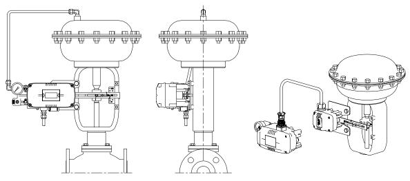
Fig. 3-2: YT-2500L / 2550L installation example
