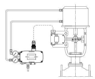
Fig. 4-7: Double acting linear actuator (YT-2501L)
