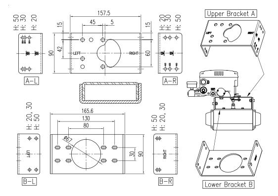
Fig. 3-14: YT-2500R / 2550R Brackets and positioner
