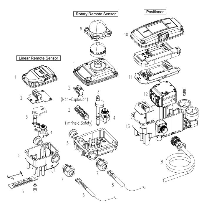
Fig. 2-2: YT-2501 exploded view
