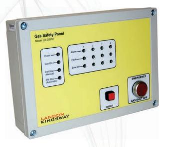
The Natural Gas Detector and LPG detector will go into alarm at 10% of the low explosion level (LEL). The Carbon Monoxide will go into alarm when the level has reached 50ppm for over 4 minutes.
