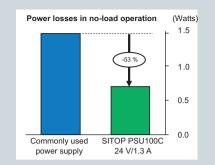
Industrial power supplies are not usually operated for 24 hours a day over the entire year. During nonproductive periods, and at weekends or holidays, individual loads or plant sections are increasingly switched to a type of "standby operation" to save energy. The SITOP PSU100C supports this with especially low no-load losses and thus with energy savings of up to 53%.
