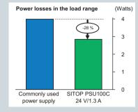
Power supplies in industrial applications are usually dimensioned to their maximum load, such as switching on capacitive loads. In operation, they are mainly run only within a load range of 30% to 70% of rated power – dependent on the process, e.g. switching motors, sensors and actuators. Because of this, the high efficiency of the SITOP PSU100C across the entire load range permits energy savings of up to 28%.
