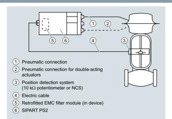
Separate installation of the position detection and positioner SIPART PS2
