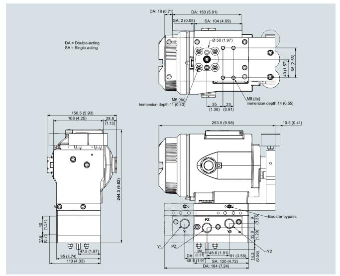
Booster mounted on positioner in a flame proof enclosure, dimensions in  $\operatorname{mm}$  (inch)
