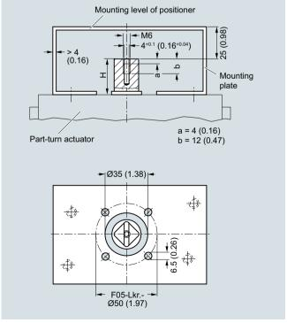
Mounting onto part-turn actuators; mounting console can be ordered via 6DR4004-1D/-2D/-3D/-4D, extract from VDI/VDE 3845, dimensions in mm (inch)
