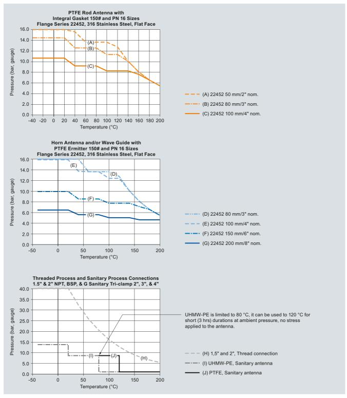
SITRANS LR200 Process Pressure/Temperature derating curves
