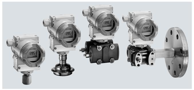
SITRANS P DS III pressure transmitters are digital pressure transmitters featuring extensive user-friendliness and high accuracy. The parameterization is performed using control keys or via HART communication, PROFIBUS-PA or FOUNDATION Fieldbus interface.
