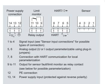
Connection diagram for power supply, input and outputs
