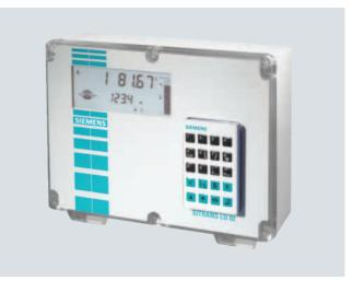
The SITRANS LU02 is a dual point ultrasonic long-range level controller for liquids and solids in one or two vessels up to 60 m (200 ft).
