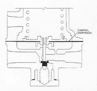
If downstream pressure increases above setpoint, the increased pressure is transmitted through the aspirator tube to the underside of the control diaphragm. The force due to downstream pressure acting on the diaphragm area will move the diaphragm up allowing the supply valve to be seated. As the diaphragm continues to move up, the relief seat will lift away from the end of the pintle, allowing downstream air to be vented, thus reducing pressure.
