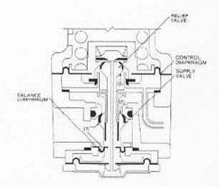
When set point is reached, the force acting on the bottom of the control diaphragm is in balance with the force acting on the top of the control diaphragm. At this point the force (1) due to supply pressure acting on the supply valve and the force (1) due to supply pressure acting on top of the balance diaphragm are in balance. The force (2) due to
