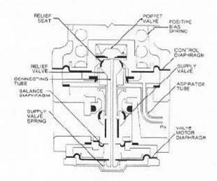
When the knob of the regulator is adjusted to a specific set point, the positive bias spring exerts a force against the top of the control diaphragm. The combined force is the result of the force exercised by the positive bias spring to produce an output pressure Po = K where K is the spring constant. This force will keep the relief seat against the
