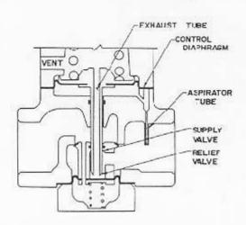
ing on the top of the supply valve is balanced by force (2) due to downstream pressure acting on the bottom of the balance diaphragm, if the downstream pressure increases, the increased pressure will be sensed on the underside of the diaphragm through the aspirator tube, and the diaphragm will move upward, seating the supply valve. As the diaphragm continues to move
