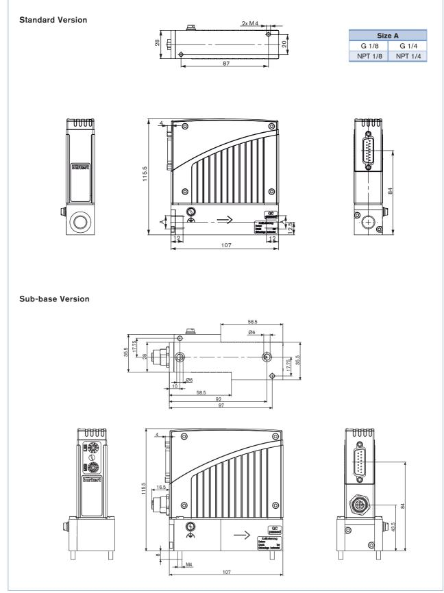
In devices without fieldbus communication there is no electrical M12 connector in the upper housing part.
