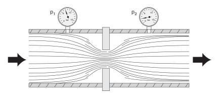
To avoid a blockage of the aperture by contaminated mediums an upstream filter is recommended.
