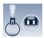
The E-shaped magnetic system inside the sensor induces a magnetic field into the fluid, which is perpendicular to the direction of flow.
