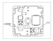
The electronics Type 2508 LR is used for power reduction of solenoid valves. Therewith the power consumption and the coil temperature can be reduced considerably e.g. with continuous operation. The inrush power conforms at this juncture to the nominal power of the coil. After switching the valve the electronic decreases to a small holding capacity. In holding operation the function is displayed by a yellow LED.
