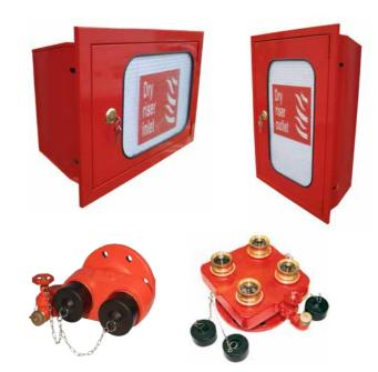
Landing valves for dry and wet riser systems, housed in outlet cabinets and manufactured by Landon Kingsway in accordance with BS5041, provide an outlet connection via BS336 coupling to each floor except ground.
