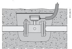
Figure 5-3 Direct burial of sensor
