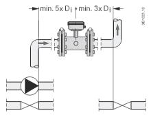
Figure 4-5 Inlet and outlet conditions
