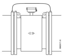
Figure 4-10 Cathodic protection
