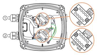
5. Connect the coil and electrode cable shields and grounding cables to the terminal board by using grounding lugs.
