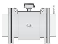
Figure 4-9 Potential equalization with grounding electrodes
