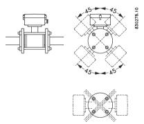
Figure 4-8 Horizontal installation, various terminal box positions
