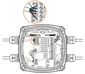
Figure 5-2 Electrode cable with individual wire shields
