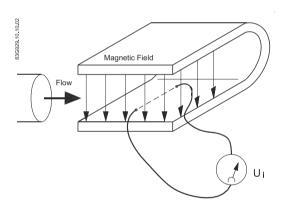
$U_i$  = When an electrical conductor of length L is moved at velocity v, perpendicular to the lines of flux through a magnetic field of strength B, the voltage  $U_i$  is induced at the ends of the conductor
