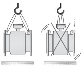
Figure 6-1 Handling of sensor
