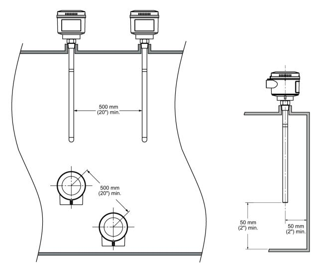
Horizontally mounted units are configured as point level switches. Mount diagonally if vertical space is restricted.
