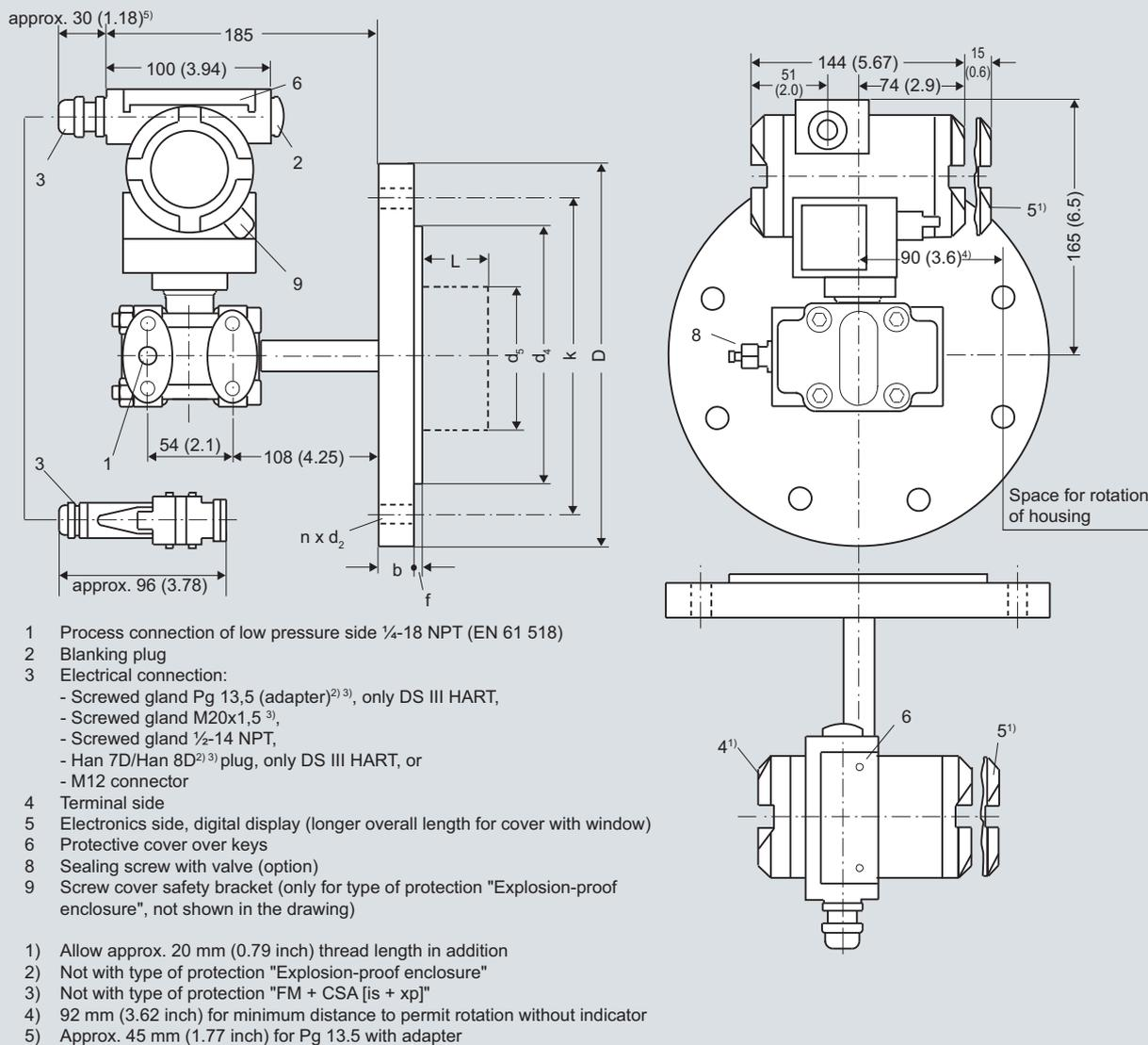
SITRANS P DS III HART pressure transmitters for level, including mounting flange, dimensions in mm (inch)
