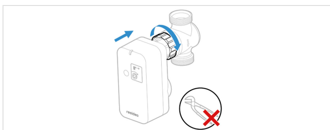
Fig. 3 Mounting the actuator
