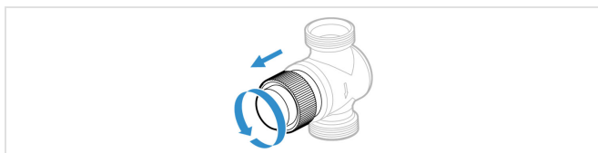
Fig. 2 Removing protection cap
