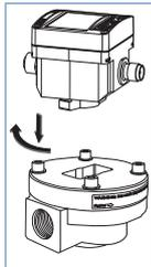
The 8072 flow sensor / switch is built up with an SE32 electronic module associated to a fitting S070 with integrated measurement oval rotor. The output signal is provided via cable plug according to EN 175301-803 and/or a M12 multipin connector.
