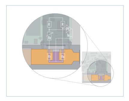
This sensor works as a hot-film anemometer in the so-called CTA operational mode (Constant Temperature Anemometer). To do this, two resistors with precisely specified temperature coefficients are located directly in the media flow and three resistors are located outside the flow are connected together to form a bridge.
